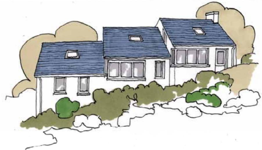
A slope can be accommodated without altering the ground, simply by changing the internal floor levels to suit. Seek a naturally flat site or cut into the hillside. Try to orientate the building with the contours to give an integrated appearance with the land, provide shelter and warmth, and reduce energy loss due to exposure.
