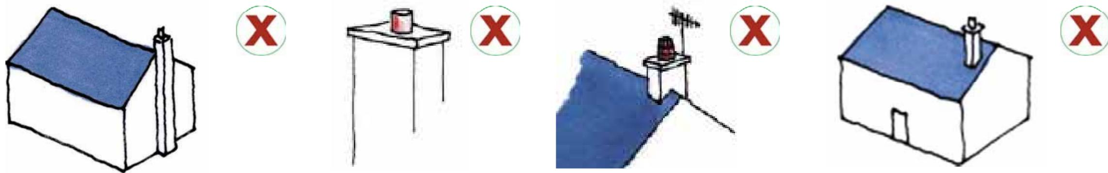
Avoid tall, spindly types positioned on the pitch of the roof as per the examples set out above
