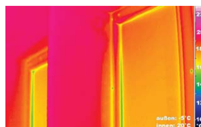
Infrared image of the interior of a passive house window. All surfaces (wall structure, window frame, and the glazing) are pleasantly warm (over 17°C). Even at the glass edge, the temperature does not fall below 15°C (light green area).
